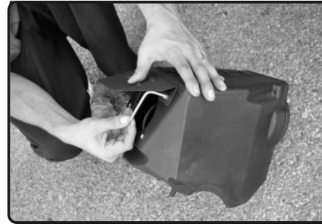
3. Use an allen wrench and remove the Air Box Shield Air Director from the Injen air box. This shield will no longer be used when installing the Injen EVO15069 Scoop
