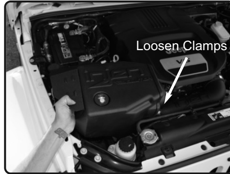
2. Loosen the clamp on the 4.0" hump hose and remove the Injen intake box from the engine bay.
