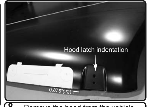
8. Remove the hood from the vehicle. Measure 0.875" (22mm) from the hood latch indentation outer tangent point. Tape the cut template onto the hood. Figure 9 will have a close up of the measuring point
