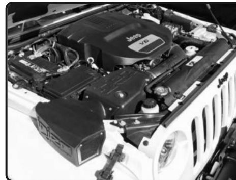
7. Injen intake system and air scoop installed.
