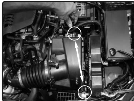
6. Loosen the two 10mm bolts holding in the stock air box. Save for later install.
