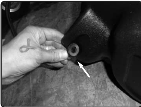
17. Remove the 2 smaller OEM grommets with crush washer from the OEM air box and install to the mounting points on injen EVO box.
