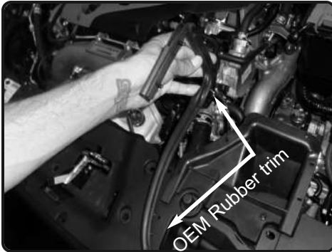
13. Remove the OEM rubber trim from the scoop using pliers. carefully pull out the clips holding in the rubber trim.
