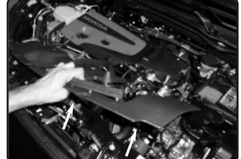
12. Remove the plastic push clips and remove the plastic radiator shroud.
