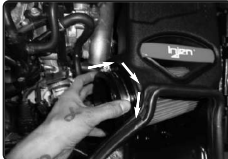
22. Once the twist lock filter is seated correctly rotate in either direction 1/4" turn untill filter locks into place.
