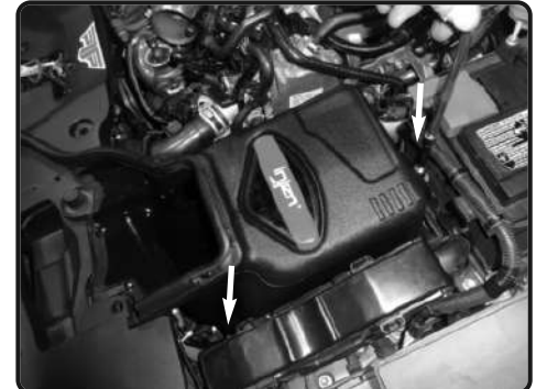
20. Once seated properly use the OEM screws from step 6, and secure the air box.
