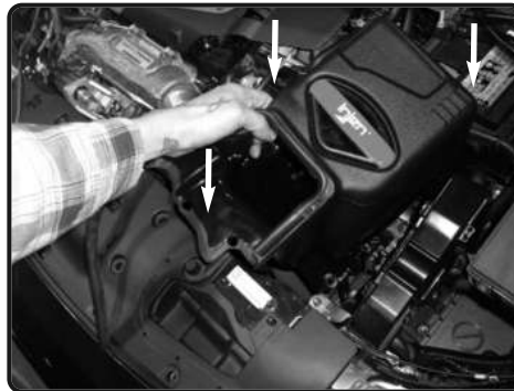
19. Install the injen EVO air box assembly into the vehicle. Position to the OEM air box locations.
