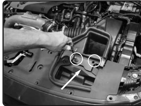
2. Loosen the 2 bolts holding in the OEM rubber Ram scoop.
