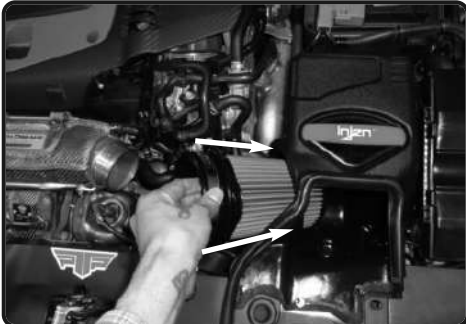
21. Install the injen twist lock filter into the air box.
