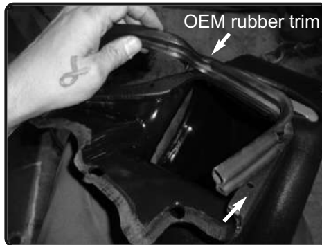
15. Install the OEM rubber trim to the injen EVO air box.
