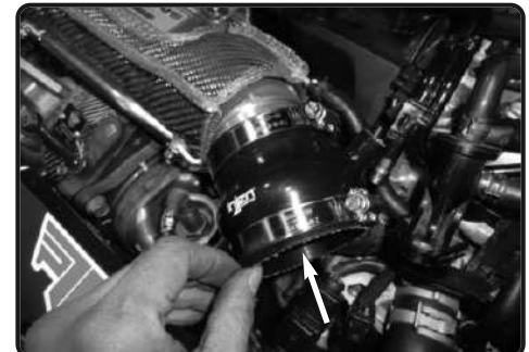
24. Install the step hump hose with clamps provided to the throttle body and position. Do not tighten.
