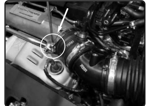
8. Loosen the clamp on turbo using phillips screwdriver.
