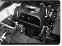
**12.** Install the air box into vehicle and position to OEM location.
