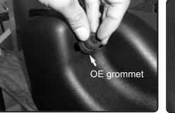
**9.** Install the OEM grommet to the hole on the air box.
