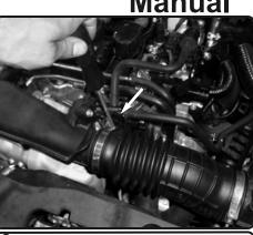
**2.** Loosen the clamp on the turbo housing using either a phillips screwdriver or 5.5mm socket.
