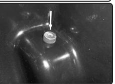
**10.** Now install the crush washer inside air box to the grommet.
