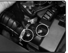
**4.** Loosen the 2 screws holding in the MAF sensor and remove. Save screws for later install.
