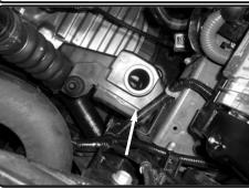
**11.** Locate the resonator box hole, make sure the OEM grommet is installed and seated properly.
