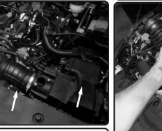
6. Pull back the intake tube from turbo housing.
