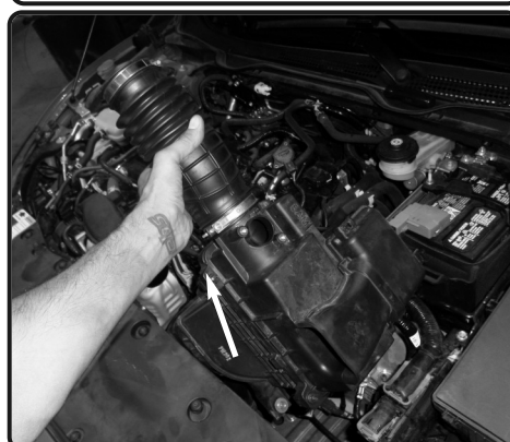
7. Now carefully lift up and remove the stock intake out of the vehicle.
