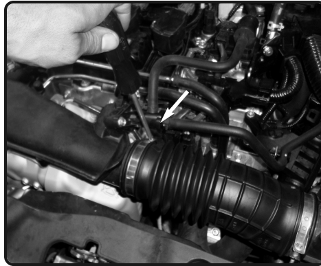
2. Loosen the clamp on the turbo housing using either a phillips screwdriver or 5.5mm socket.
