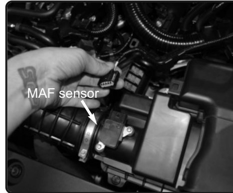
3. Disconnect the MAF sensor.
