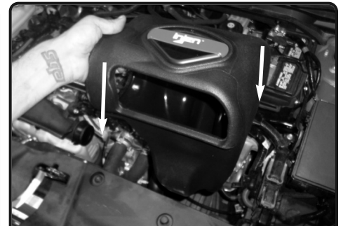
12. Install the air box into vehicle and position to OEM location.
