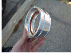
8. Install the O-ring onto the billet machined adapter. Make sure to install it in the same direction as the OEM tube.
