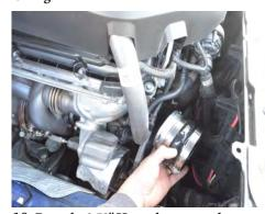
10. Press the 3.50" Hump hose on to the billet machine adapter then secure it using the provide clamps.
