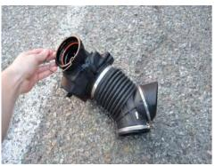
6. Remove the OEM retaining clip from the tube. It will be reused on the Injen intake.
