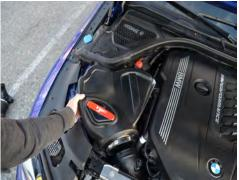
17. Install the twist lock filter on to the Injen air 16. Install the Injen air box into the engine bay. Line up the studs on the air box to the factory grommets and press down on the box.
