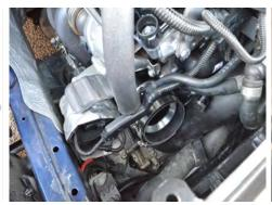
11. Press the billet machined adapter on to the turbo inlet until you hear the retaining clip snap into place.
