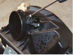
12. Remove the two screws holding the temp senor then remove the temp sensor.
