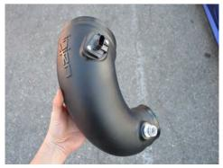
13. Install the temp sensor onto the Injen tube and secure using the provided M4 button head
