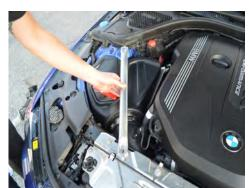
22. Reinstall the strut tower brace.
