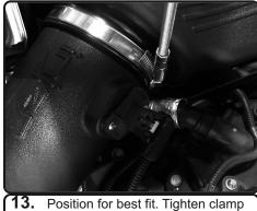
**13.** Position for best fit. Tighten clan on filter using 8mm nut driver.
