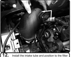
**12.** Install the intake tube and position to the filter and the tube to the turbo.
