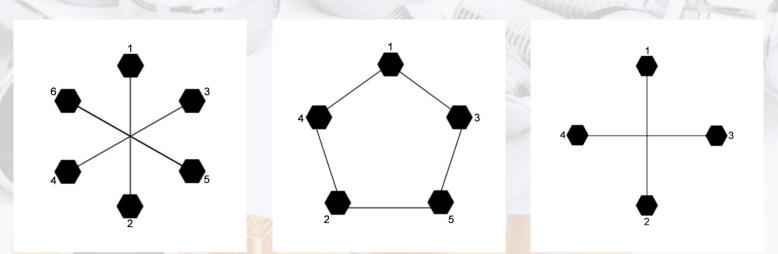
3/8" STUD DIA. – 35-45 ft/lbs 7/16" STUD DIA. – 55-65 ft/lbs 1/2" STUD DIA. – 75-85 ft/lbs 9/16" STUD DIA. – 95-115 ft/lbs 12 mm STUD DIA. – 70-80 ft/lbs 14 mm STUD DIA. – 85-95 ft/lbs
