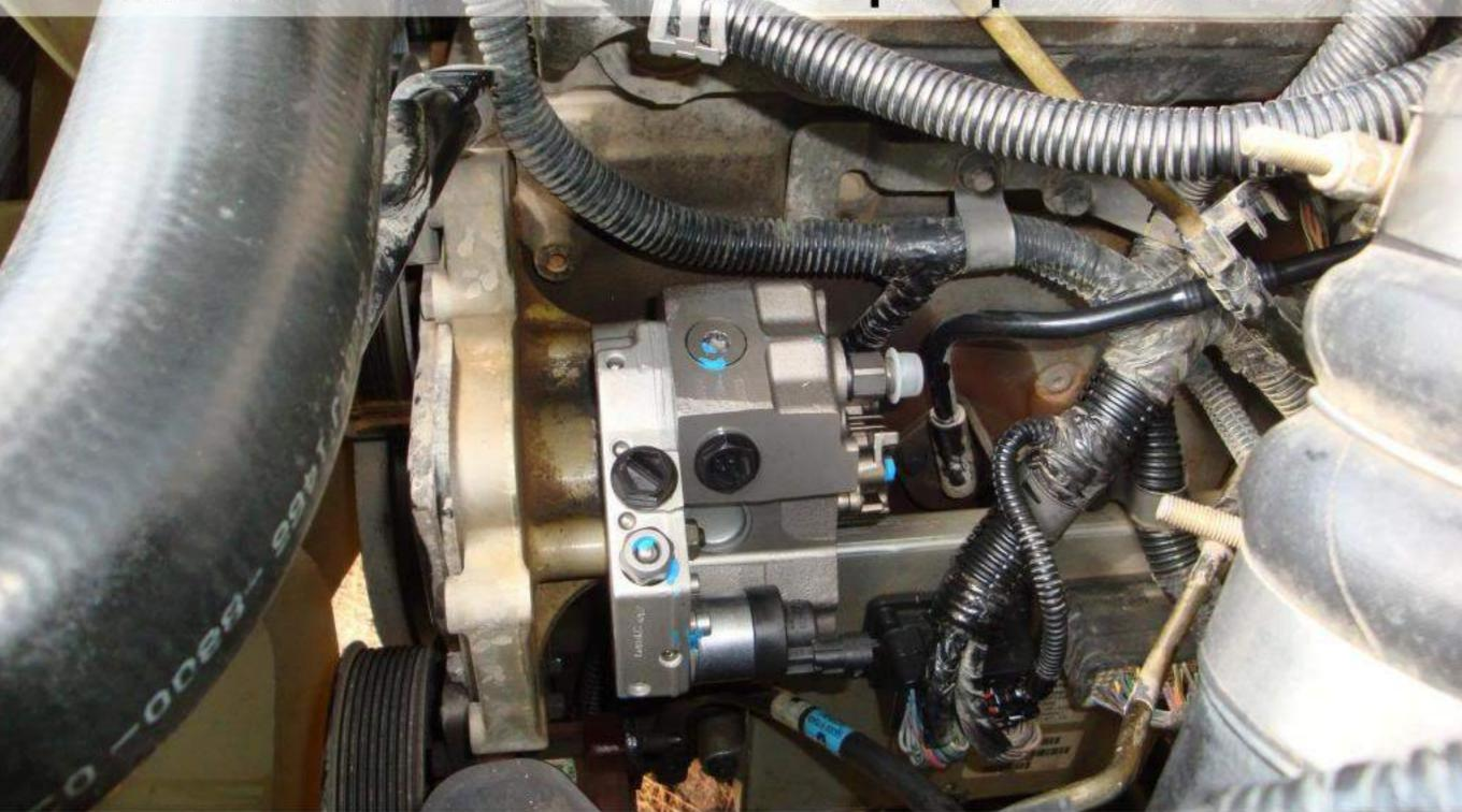
Once the nuts are tight, tighten the pump gear nut to 77 ft/lbs.
