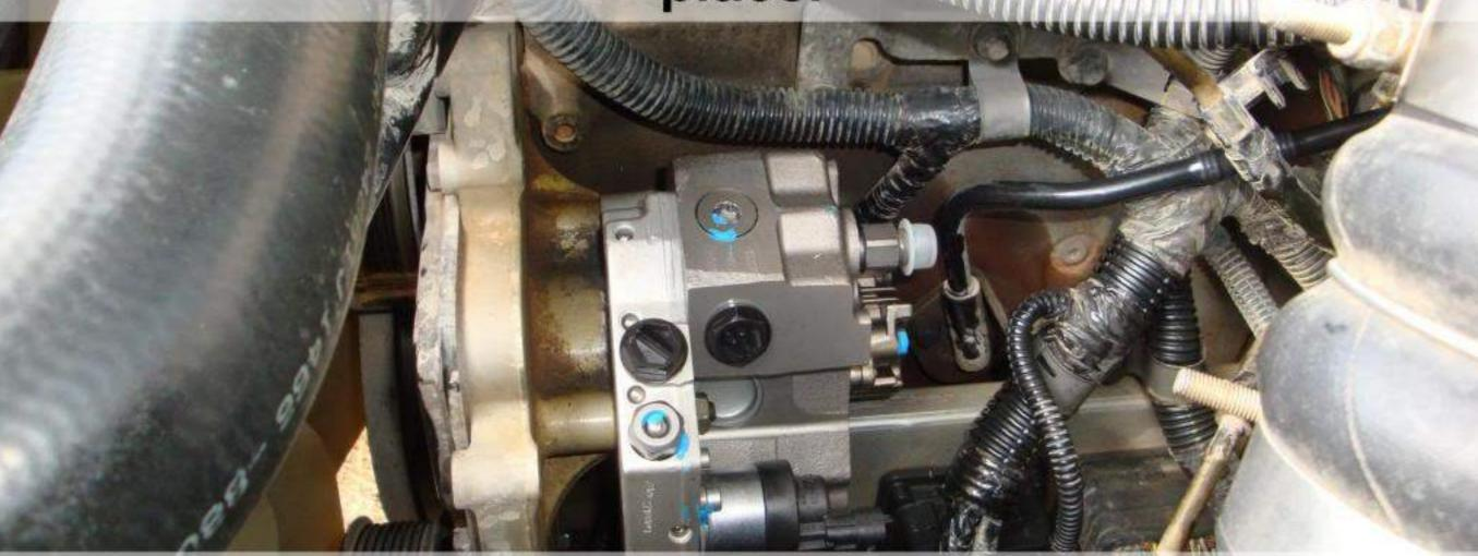
Once the pump is in place, finger tighten the three 13mm nuts. Once these are finger tight, use a 27mm socket to lightly tighten the pump gear nut to the shaft.
