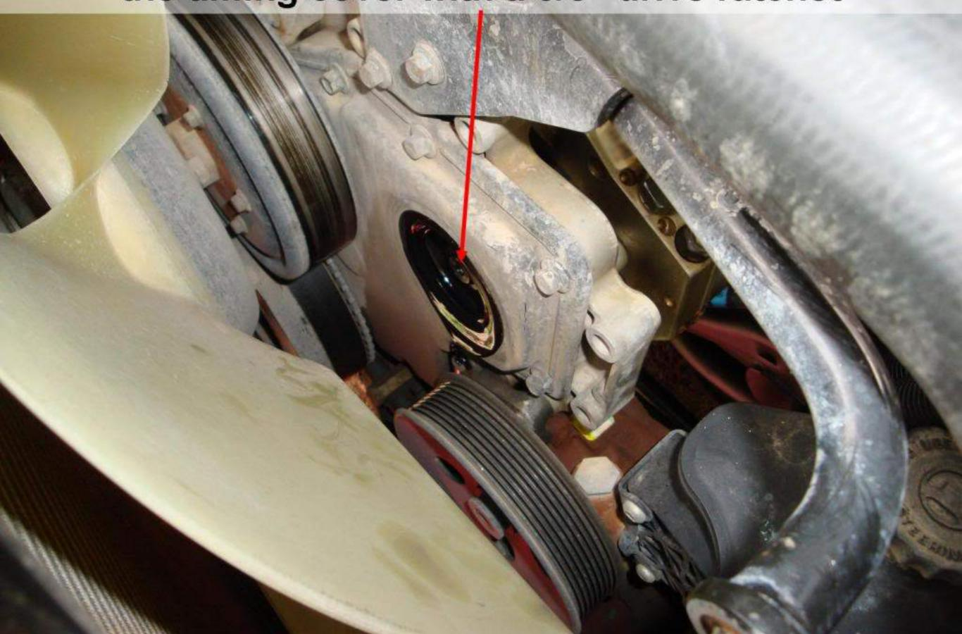
Remove the pump gear from the pump shaft with a small gear puller. Leave the gear in the housing with the puller attached.
