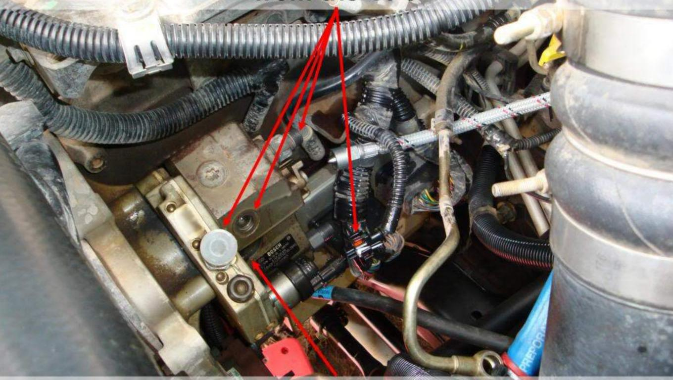
Remove the three 13mm nuts securing the CP3 to the pump mounting stude
