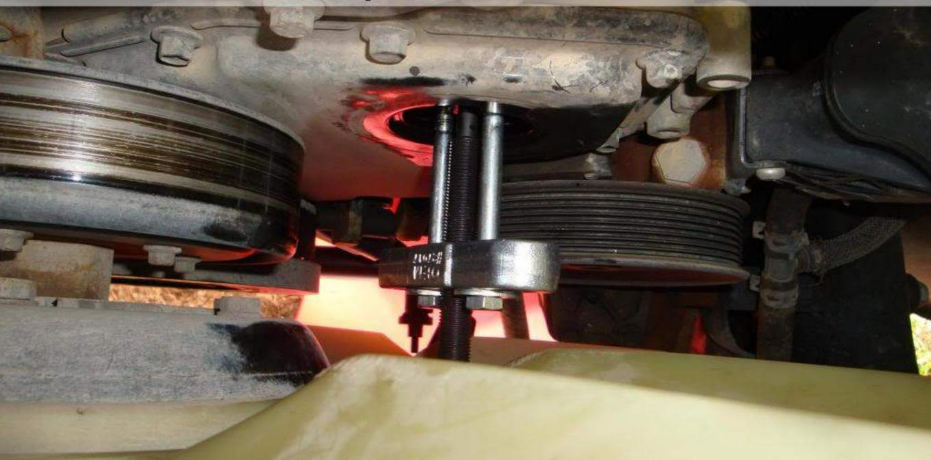
Once the pump gear is removed from the shaft, you can pull the CP3 out from the back.
