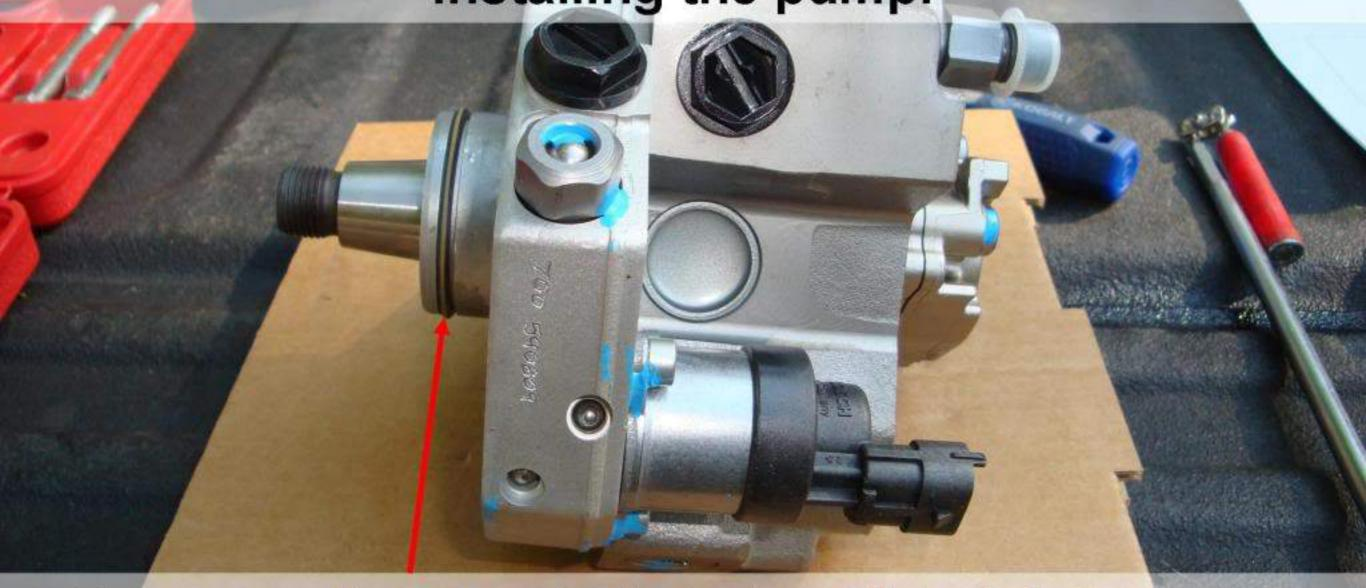
Use a small amount of engine oil to lubricate the new seal and pump pilot before installing the new pump. DO NOT lube the pump shaft.
