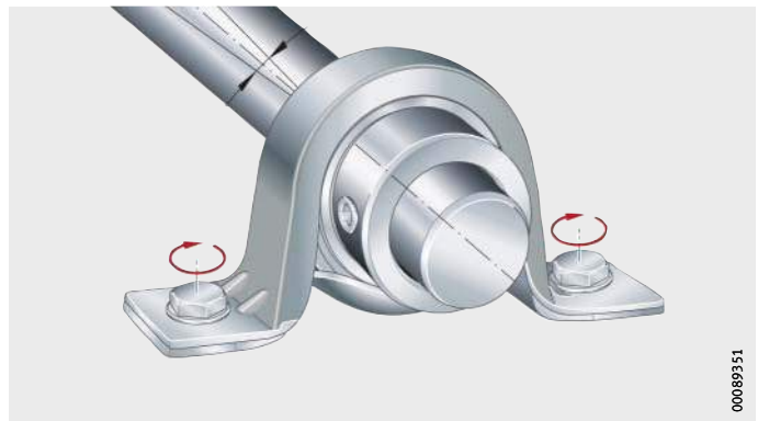
Figure 12 Screw mounting the housing finger tight
