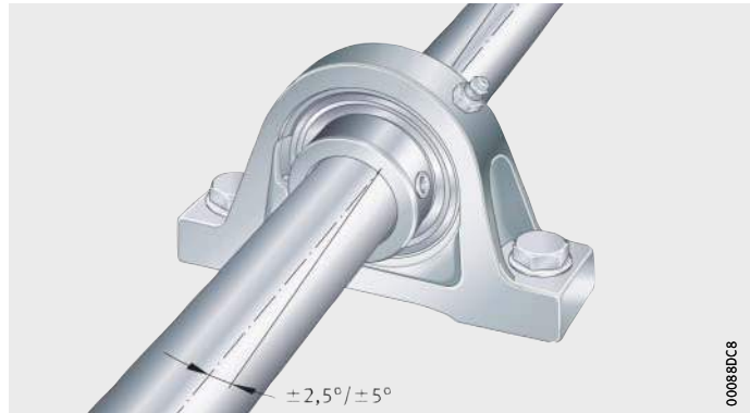
Figure 5 Compensation of static shaft misalignment
