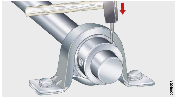
Figure 13 Tensioning the eccentric locking collar
