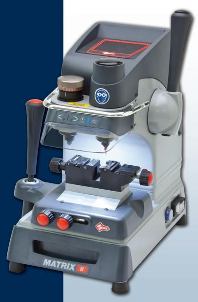
The Matrix II is a high performance machine that provides precision duplication of laser style keys. The features of this premium model include LED lighting and electromechanical calibration. The compact design and weight make this model suitable for either counter or mobile use.
