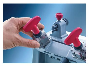
**Optimized calibration** A tracer point adjustment system provides fast, precise calibration.
