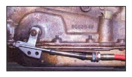
13. Try to shift the column. You may experience a tight pattern, if so slightly loose the bracket around the column. This should allow the column to move easier. If not check that the cable is in alignment from the bracket to the lever.
