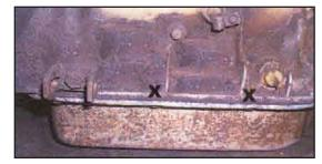
10. The two transmission pan bolts could be either Metric or American threads. You will need to purchase two bolts 1/4" longer
