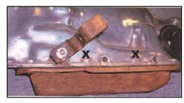
10. The two transmission pan bolts could be either Metric or American threads. You will need to
