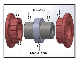
18. Install the ICON UCA into position and slide the factory mounting bolt through the bushings and frame. Apply thread locker to the threads of the bolt and install the nut (passenger side shown). [FIGURE 17 & 18]
