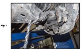
2. Touch up drilled hole with paint to avoid corrosion.
