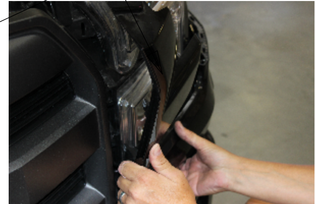
Step 4 Headlight surround removal
