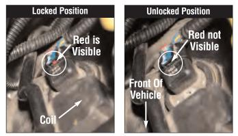
Disconnect the factory connector for the 4-Pin cam sensor. This connector has a locking clip that must be slid back to unlock. Notice the slight difference in the position when the tab is in the "UNLOCKED" position. Then, squeeze down the locking tab, and push the connector in slightly (toward sensor) and then remove.
