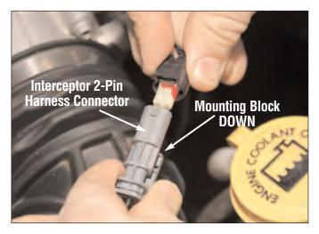
Plug the Interceptor harness 2-Pin connector into the factory wiring harness 2-Pin connector. *NOTE: The correct orientation of the connector is shown above (mounting block DOWN).*
