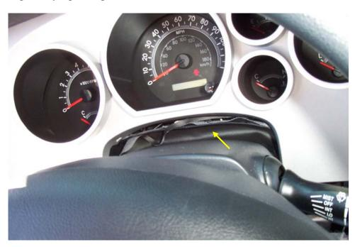
d. Utilizing the openings in the bezel, use your fingers to press the locking mechanisms to release the curtain from the bezel.
