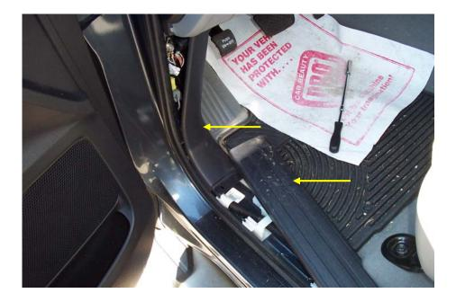
3. Using a 10mm tool, remove the bolts from the lower IPC (Instrument Panel Cluster) trim bezel.
