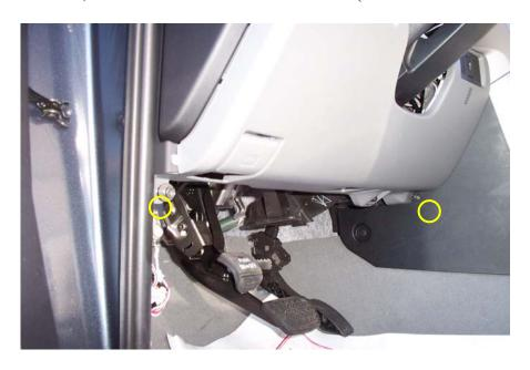
4. Starting on the left hand side, gently separate the lower IPC trim bezel, from the dash, and lower it to the floorboard.
