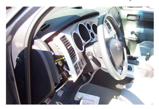
b. While peering behind the upper IPC panel bezel, you will need to disconnect two connectors. **Note:** To prevent breaking the connectors, **DO NOT rock the connector** back and forth. Squeeze the release and pull straight out.
