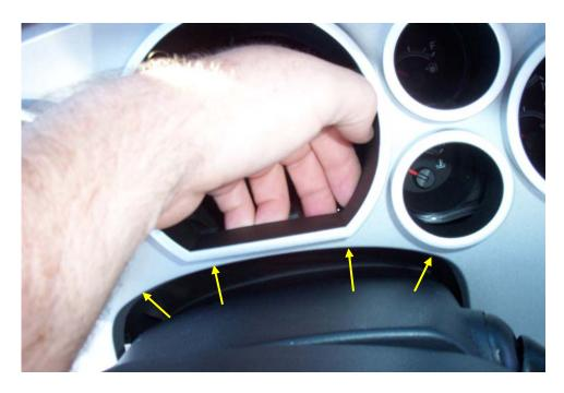
6. Utilizing a 10mm tool, remove the retaining bolts from the IPC. Pull the unit forward and disconnect it from the harness. **Note: To prevent breaking the connectors, DO NOT rock the connector back and forth. Squeeze the release and pull straight out.**
