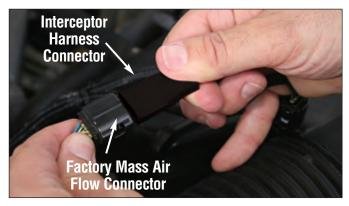
Plug the Interceptor harness connector into the factory Mass Air Flow connector.
