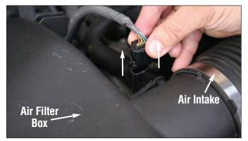
Disconnect the factory connector from the Mass Air Flow sensor. Push down on the connector, squeeze the release tab firmly, then pull up to remove the connector.
