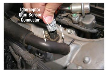
Plug the Interceptor Cam sensor connector into the Cam sensor.
