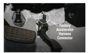
Using a flashlight, locate the factory accelerator harness connector under the driver's dashboard and above the accelerator pedal. Disconnect the factory harness from the accelerator pedal sensor by pushing down on the connector, squeezing the release tab firmly, then pulling up to remove the connector.
