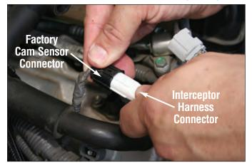
Plug the Interceptor harness connector into the factory Cam sensor connector.
