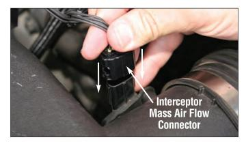
Plug the Interceptor Mass Air Flow sensor connector into the vehicle Mass Air Flow sensor.
