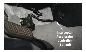
Tuck the Interceptor accelerator controller behind the carpet and console and out of the way of the accelerator pedal, making sure all other wires/connectors are out of the way of the accelerator pedal as well. Installation is now complete! You are now ready to enjoy more power and performance with the Hypertech Interceptor!
