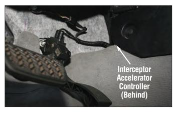
Tuck the Interceptor accelerator controller behind the carpet and console and out of the way of the accelerator pedal, making sure all other wires/connectors are out of the way of the accelerator pedal as well. Installation is now complete! You are now ready to enjoy more power and performance with the Hypertech Interceptor!
