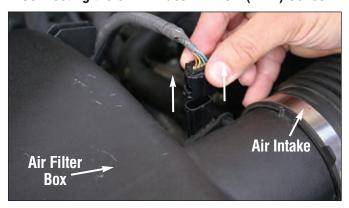
Disconnect the factory connector from the Mass Air Flow sensor. Push down on the connector, squeeze the release tab firmly, then pull up to remove the connector.
