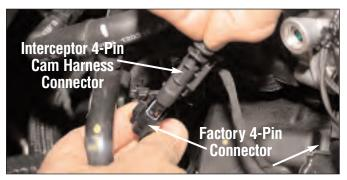
Plug the Interceptor 4-Pin cam harness connector into the factory wiring harness 4-Pin connector.
