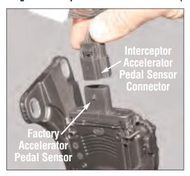
Plug the Interceptor accelerator pedal sensor connector into the factory accelerator pedal sensor.
