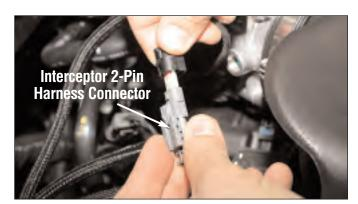
Plug the Interceptor harness 2-Pin connector into the factory wiring harness 2-Pin connector. **NOTE: The correct orientation of the connector is shown above.**
