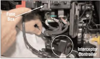
Place Interceptor Controller on its side in the compartment, making sure no cables are pinched or bent. Then re-install the fuse box back to its original location.
