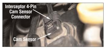
Plug the Interceptor 4-Pin cam sensor connector into the vehicle cam sensor.
