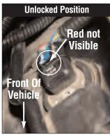
Disconnect the factory connector from the 4-Pin cam sensor. This connector MAY have a locking clip that must be slid back to unlock. Notice the slight difference in the position when the tab is in the "UNLOCKED" position. Then, squeeze down the locking tab, and push the connector in slightly (toward sensor) and then remove.
