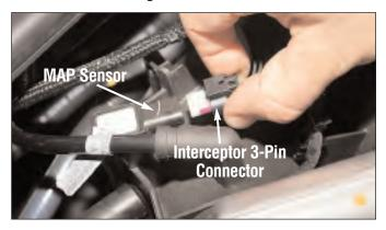
Plug the Interceptor 3-Pin connector into the vehicle MAP sensor.
