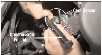
Locate the cam sensor near the transmission fill tube on the passenger side.
