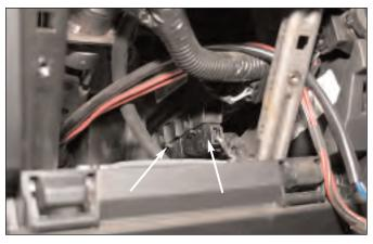
Using the 10mm socket and ratchet, remove the metal plate located behind the dash panel. Then, remove the two (2) connectors from the module behind the metal plate. Move these to the side for easier access and visibility.
