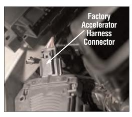
Disconnect the factory harness from the acceleratoe pedal sensor. Using a flashlight, you should see the accelerator pedal connector just behind the module which was unplugged in t he previous step. This picture is taken from the pedal area, looking up toward the windshield.
