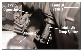
Disconnect the factory connector from the 2-Pin (intake air temp) sensor.
