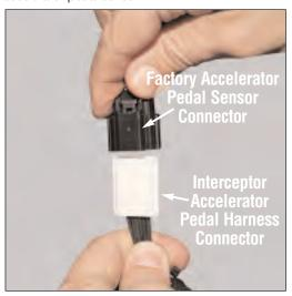
Plug the Interceptor accelerator pedal harness connector into the vehicle's factory accelerator pedal sensor connector. Position the Interceptor Accelerator Controller out of the way of the accelerator. Reinstall the two (2) connectors to the module behind the dash panel and the metal plate removed from Step 2, then reinstall the dash panel removed in Step 1. Installation is now complete.
