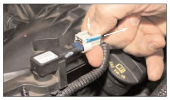
Disconnect the factory connector for the 3-Pin (MAP) sensor. This connector has a locking clip that must be slid back to unlock. Then, squeeze down the locking tab, and push the connector in slightly (toward sensor) and then remove.
