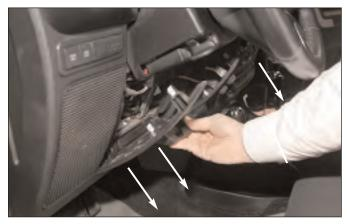
Remove the dash panel below the steering wheel by pulling back at the top of the panel. This will allow for easier access and visibility when installing the Interceptor Accelerator Controller.
