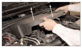
Lift off the engine cover and place it to the side while installing the Hypertech Interceptor.
