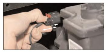
Disconnect the factory connector from the MAP sensor. This connector has a locking clip that must be slid back to unlock. Then, squeeze down the locking tab, and push the connector in slightly (toward sensor) and then remove.
