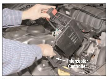
Place Interceptor Controller on its side in the compartment. Then re-install the fuse box back to its original location.
