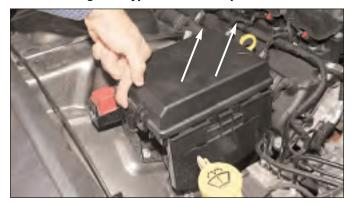
Locate fuse box in the engine compartment on the passenger side. Press the locking tabs to disengage fuse box and lift up to expose empty compartment. Locking tabs may vary slightly from those shown above.
