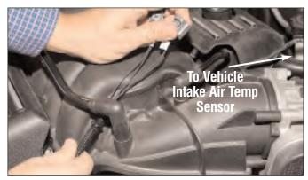
Route the Interceptor wire to vehicle intake air temp sensor.
