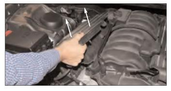
Lift off the passenger side engine cover.
