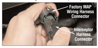
Plug the Interceptor harness connector into the factory MAP wiring harness connector, and push in the locking clip.
