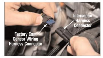
Plug the Interceptor harness connector into the factory cam sensor wiring harness connector.
