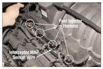
Route the Interceptor MAP sensor harness under the fuel injector harness to the MAP sensor. (SRT8 engine show for clarity ONLY).
