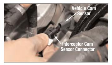
Plug the Interceptor cam sensor connector into the vehicle cam sensor.
