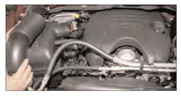
Using a flathead screwdriver, loosen the clamp at air filter box and lift the intake hose out of the way.
