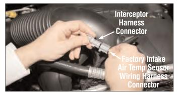
Plug the Interceptor harness connector into the factory intake air temp sensor wiring harness connector.
