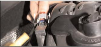
Disconnect the factory connector from the 3-Pin MAP sensor. This connector has a locking clip that must be slid back to unlock. Notice the slight difference in the position when the tab is in the "UNLOCKED" position. Then, squeeze down the locking tab, and push the connector in slightly (toward sensor) and then remove.
