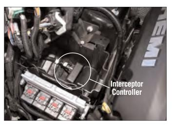
Place Interceptor Controller on its side in the compartment, making sure no cables are pinched or bent. Then re-install the fuse box back to its original location.
