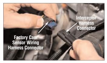
Plug the Interceptor harness connector into the factory cam sensor wiring harness connector. **NOTE: The correct orientation of the connector is shown above.**
