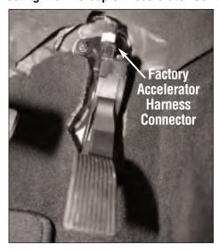
Using a flashlight, locate the factory accelerator harness connector under the driver's dashboard and above the accelerator pedal. Push the carpeted compartment cover out of the way if necessary so you can disconnect the factory harness from the accelerator pedal sensor.
