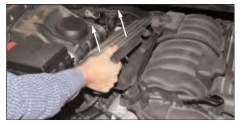
Lift off the passenger side engine cover.
