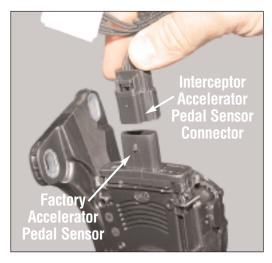
Plug the Interceptor accelerator pedal sensor connector into the factory accelerator pedal sensor.
