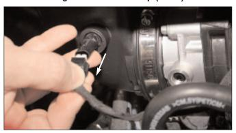
Disconnect the factory connector from the 2-Pin (Intake Air Temp) sensor. Next, plug the Interceptor 2-Pin connector into the vehicle Intake Air temp sensor.
