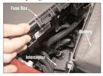
Locate fuse box in the engine compartment on the driver's side. Press the locking tabs to disengage fuse box and lift up to expose empty compartment. Locking tabs may vary slightly from those shown above. Place Interceptor Controller as shown and route the Interceptor cable out of the existing channel. Then re-install the fuse box back to its original location.
