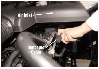
Route the Interceptor harness between the throttle body and air inlet pipe, and then back to the 4-Pin (CAM) sensor.
