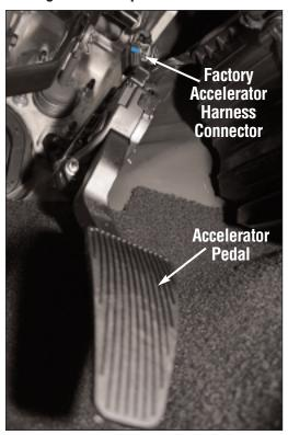
Using a flashlight, locate the factory accelerator harness connector under the driver's dashboard and above the accelerator pedal. Disconnect the factory harness from the accelerator pedal sensor.
