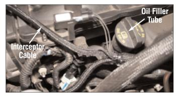
Route the Interceptor harness and all connectors away from the oil fill tube, and hold in place with provided zip-ties as necessary.
