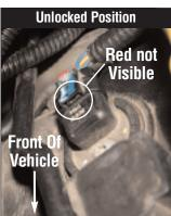
Disconnect the factory connector for the 4-Pin cam sensor. The Cam sensor is located on the passenger side behind the air intake tubing (See above photo). This connector has a locking clip that must be slid back to unlock. Notice the slight difference in the position when the tab is in the "UNLOCKED" position. Then, squeeze down the locking tab, and push the connector in slightly (toward sensor) and then remove.
