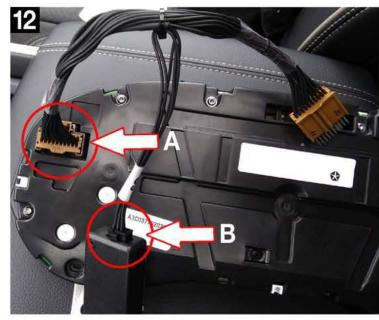
13. Plug in the male connector of the Hypertech In-Line Speedometer Calibrator Module harness to the connector on the vehicle harness, taking care to match like sides of the connectors. Secure the harness connectors with the supplied zip tie as shown.
