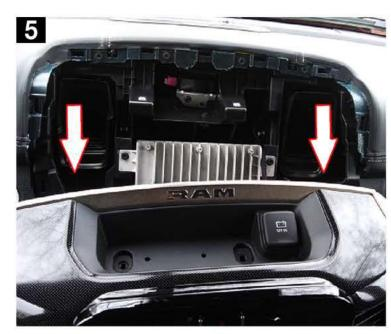
This step is for the Ram 1500 ONLY. Remove the lower knee panel directly under the steering wheel by removing the two (2) 7mm bolts. Pull the panel toward the rear of the truck to release the tabs holding the panel in place.
