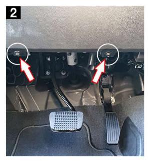
Pull the kickplate back toward the driver seat to release the clips holding it in place.
