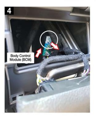
5. Plug the female connector of the In-Line Speedometer Calibrator Module harness into the BCM (Pic 5A). Then plug the male connector of the In-Line Speedometer Calibrator Module harness into the factory connector removed from the BCM in Step 4 (Pic 5B). Make sure you hear the female connector click into place on the BCM. This can require you to push the connector pretty hard into the BCM.
