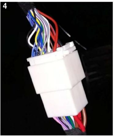
Install the In-Line Speedometer Calibrator Module under the driver's side dash, near the brake pedal. Secure the In-Line Speedometer Calibrator Module in place and tuck it up out of the way of movement in the foot well as shown.
