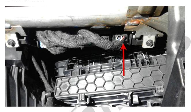
5. Insert the male connector of the speedometer harness into the factory vehicle harness, making sure to align the connectors so that both the retaining clips are facing up. Secure the 2 connectors with a zip-tie through the retaining clips. Be sure to not pull the zip-tie too tight to avoid damage to the clips.
