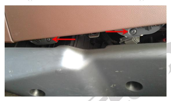
3. Open the glove box and remove the (2) T15 Torx screws at the top. There are a few clips on the backside that retain the glove box, pull gently towards yourself and it will come free.
