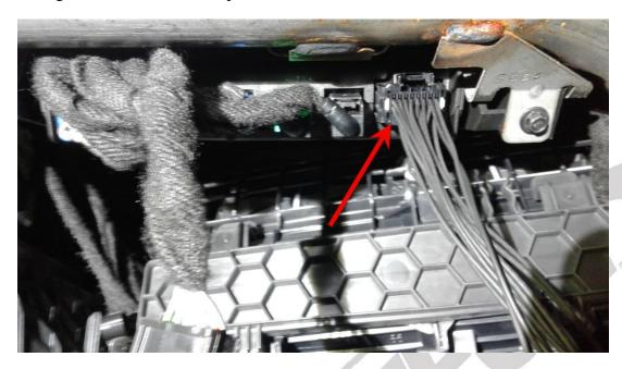
7. Place the speedometer calibrator module and harness in the area behind the vehicle's module and secure it with a zip-tie.
