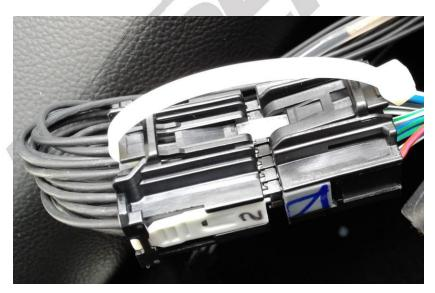
6. Plug the female end of the speedometer calibrator harness into the module.
