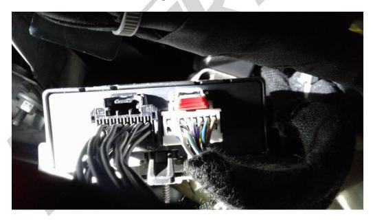
7. Tuck the harness up in front of the module, it should rest nicely in the area in front of the module.
