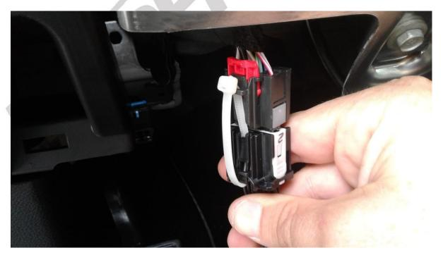
8. Plug the female end of the Speedometer Calibrator harness into the vehicle's module.
