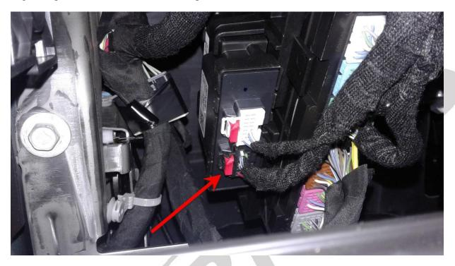
7. Insert the male portion of the Speedometer Calibrator harness into the female end of the vehicle's harness. Make sure to align the connectors so that the locking tabs are on the same side. Run a zip-tie through the tabs to secure the connectors.
