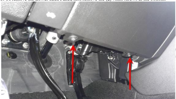
4. Pull back on the Left and Right side of the Kick Panel at the top to release it. There is one connector for the headlight switch on the left.
