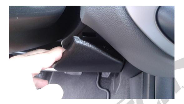
5. Depress tab on headlight switch connector and pull back to disconnect.
