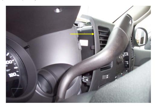
2. Using a trim removal tool, or your fingers, carefully separate the Left-hand Console Bezel.
