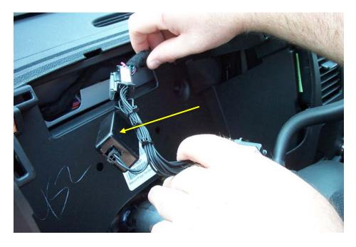
d. Stow the harness assembly, except for C1, into the back area as shown below.
