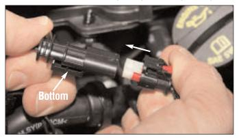
Plug the Interceptor harness connector into the factory 3-Pin sensor wiring harness connector. *NOTE: The correct orientation of the connector is shown. This connector has a locking clip that must be slid back to lock (refer to Step1).*
