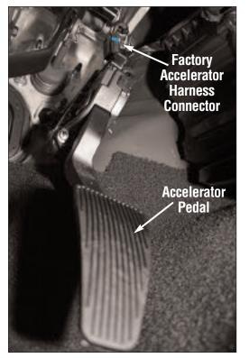
Using a flashlight, locate the factory accelerator harness connector under the driver's dashboard and above the accelerator pedal. Disconnect the factory harness from the accelerator pedal sensor.
