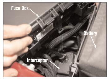
Locate fuse box in the engine compartment on the driver's side. Press the locking tabs to disengage fuse box and lift up to expose empty compartment. Locking tabs may vary slightly from those shown above. Place Interceptor Controller as shown and route the Interceptor cable out of the existing channel. Then re-install the fuse box back to its original location.
