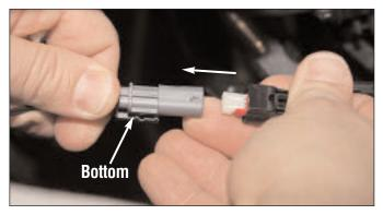
Plug the Interceptor harness 2-Pin connector into the factory wiring harness 2-Pin connector. *NOTE: The correct orientation of the connector is shown.*
