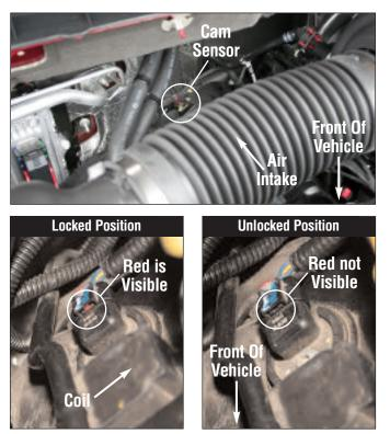
Disconnect the factory connector for the 4-Pin cam sensor. The Cam sensor is located on the passenger side behind the air intake tubing (See above photo). This connector has a locking clip that must be slid back to unlock. Notice the slight difference in the position when the tab is in the "UNLOCKED" position. Then, squeeze down the locking tab, and push the connector in slightly (toward sensor) and then remove.
