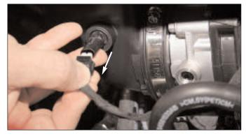
Disconnect the factory connector from the 2-Pin (Intake Air Temp) sensor. Next, plug the Interceptor 2-Pin connector into the vehicle Intake Air temp sensor.
