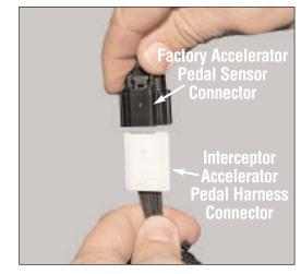
Plug the Interceptor accelerator pedal harness connector into the vehicle's factory accelerator pedal sensor connector. Position the Interceptor Accelerator Controller out of the way of the accelerator. Installation is now complete.
