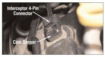
Plug the Interceptor 4-Pin connector into the vehicle cam sensor. Then plug the Interceptor harness 4-Pin connector into the factory wiring harness 4-Pin connector.
