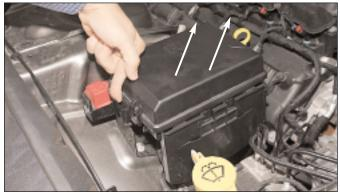
Locate fuse box in the engine compartment on the passenger side. Press the locking tabs to disengage fuse box and lift up to expose empty compartment.
