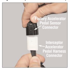
Plug the Interceptor accelerator pedal harness connector into the vehicle's factory accelerator pedal sensor connector.
