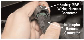
Plug the Interceptor harness connector into the factory MAP wiring harness connector, and push in the locking clip. **NOTE for Ram Truck Specific: Reposition the intake hose and use an 8mm socket to tighten the clamp at the throttle body.**
