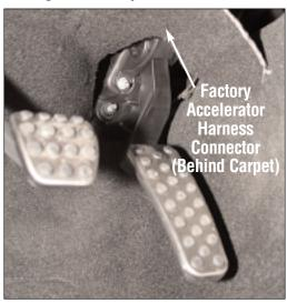
Using a flashlight, locate the factory accelerator harness connector under the driver's dashboard and above the accelerator pedal. Push the carpeted compartment cover out of the way so you can disconnect the factory harness from the accelerator pedal sensor.
