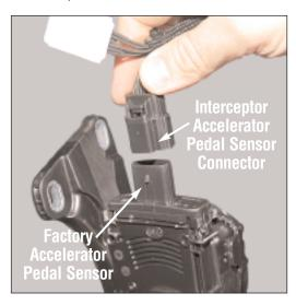
Plug the Interceptor accelerator pedal sensor connector into the factory accelerator pedal sensor.
