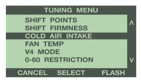
Use the buttons to the right of the screen to highlight the cold air intake installed on your vehicle. Select the Stock air intake if you have not installed an aftermarket air intake. Press 'Select' to save the chosen tune.
