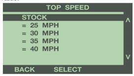
Some applications allow the top speed limiter to be lowered from the factory setting. On vehicles with this option, the initial top speed settings that appear on the programmer will LOWER the top speed from 25 to 75 MPH. Selecting one of these options will keep the vehicle from exceeding the selected speed.
