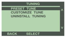
When using the programmer for the first time, select the **CUSTOMIZE TUNE** option.
