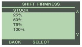
Press the 'Back' button to go back to the Gear Shift menu. Repeat the procedure above for each gear change. Once you have made the desired changes for each gear, press the 'Back' button to return to the Tuning Menu. For more information on Shift Firmness option, see Programming Features explanation in Section 4.
