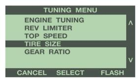
Use the buttons to the right of the screen to scroll up or down, and highlight the desired tire size, in ¼ inch increments. Press 'Select' to save the chosen value.
