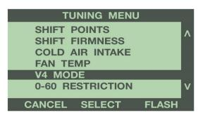
To completely disable the V4 Mode, use the buttons to the right of the screen to scroll down, and highlight Disabled. Press the 'Select' button to save this option.
