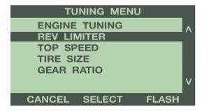
Use the buttons to the right of the screen to scroll up or down, and highlight the value to increase or decrease the engine rev limiter. Press 'Select' to save the chosen value.
