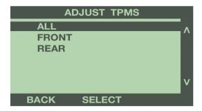
Use the buttons to the right to raise or lower the minimum tire pressure to activate the TPMS alarm. Select 'Flash' to program the change.
