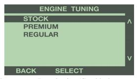
Press 'Select' to save the chosen tune. By selecting 'Stock', the programmer will install any additional features selected, but keep the stock engine tuning. For more information on Gas Engine Tuning options, see Programmer Features explanation in Section 4.
