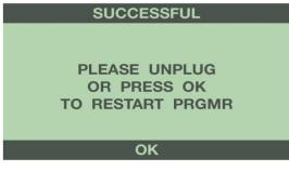
It is now safe to unplug the programmer from the vehicle and start the engine. Make sure the "Check Engine" light on the instrument cluster goes out. Warm up the engine and make sure it is running smoothly.
