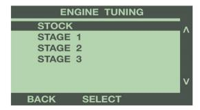
By selecting 'Stock', the programmer will install any additional features selected, but keep the stock engine tuning. For more information on Diesel Engine Tuning options, see Programmer Features explanation in Section 4.
