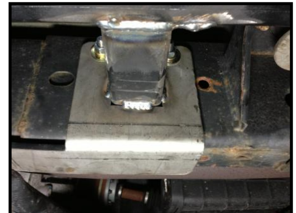
Figure 3 – U-Bolts Installed & Fastened
