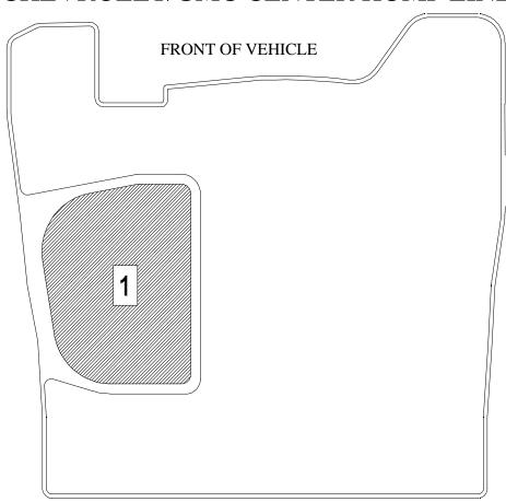
NOTE: IF YOUR VEHICLE IS EQUIPPED WITH A MANUAL SHIFT TRANSFER CASE, IT WILL BE NECESSARY TO TRIM YOUR LINER. REMOVE THE MATERIAL INSIDE OF THE RAISED BANDS (SEE AREA 1, SHOWN SHADED ABOVE). A UTILITY KNIFE OR SCISSORS WORK WELL FOR TRIMMING.
