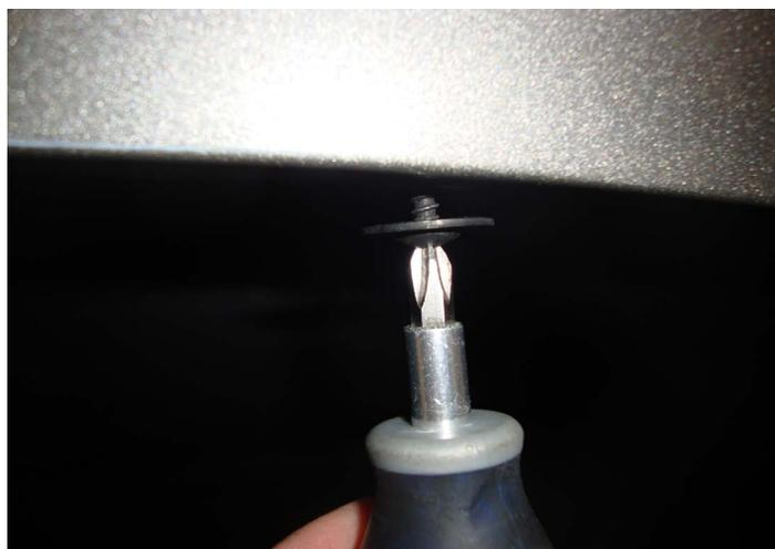
7. Align the U-Clip holes with the factory fender holes at locations B & C. Install #10 SEM screws under the fender well lip, through the fender sheet metal and into the U-Clips at location's B & C. Leave screws loose until all fasteners are installed.
