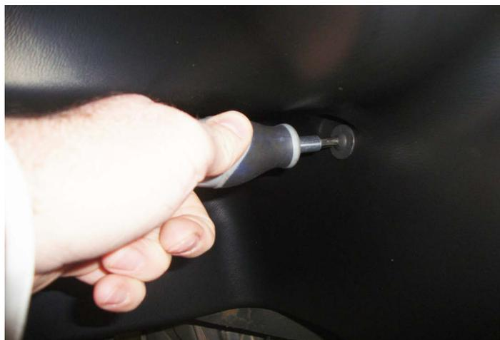
8. Install #10 SEM screws at locations A & D through the Wheel Well Guard, through the fender sheet metal and into U-Clips (see below).
