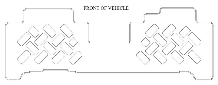
TO EASE THE INSTALLATION OF YOUR HUSKY SECOND SEAT FLOOR LINER IN YOUR FJ CRUISER, SIMPLY SLIDE BOTH FRONT SEATS TO THEIR MOST FORWARD POSITION. ONCE YOUR LINER IS INSTALLED, REPOSITION SEATS AS NEEDED.
