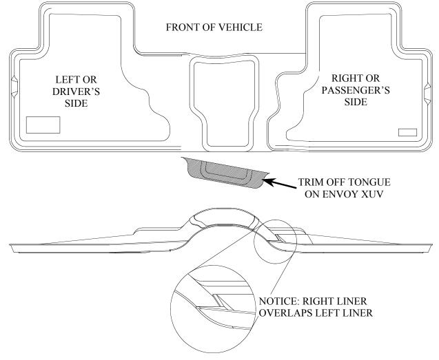
ENVOY XUV OWNERS WILL NEED TO TRIM THEIR HUSKY LINER TO ACHIEVE THE PROPER FIT. TRIM LINER AS SHOWN ABOVE USING A UTILITY KNIFE OR HEAVY SHEARS (SEE CROSSHATCHED AREA). A RECESSED TRIM GUIDE IS MOLDED IN TO AID IN TRIMMING. TRIM ALONG THE RECESS AND AGAINST THE EDGE OF THE RAISED BAND. TRIMMING PHOTOS ARE INCLUDED ON THE BACK OF THIS SHEET.
