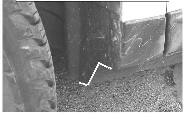
EDGE WITH OPTIONAL LOWER BODY SIDE MOLDING. NOTE MOLDING EXTENDS STRAIGHT DOWN THEN TURNS UNDER. THIS CLADDING IS COMMON ON SPORT MODELS & WITH 2.0L ECOBOOST ENGINES. IT IS OPTIONAL ON OTHER MODELS.
