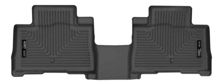
TO EASE INSTALLATION OF YOUR NEW SECOND SEAT LINER, MOVE THE FRONT ROW SEATS COMPLETELY FORWARD PRIOR TO INSTALLATION. ONCE THE LINER IS IN PLACE, MOVE THE FRONT SEATS BACK TO THE DESIRED POSITIONS.
