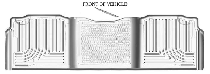
TO EASE INSTALLATION OF YOUR RAM MEGA CAB TRUCK SECOND SEAT LINER, MOVE BOTH FRONT ROW SEATS TO THEIR MOST FORWARD POSITION. WITH THIS COMPLETED, INSTALL LINER AS SHOWN IN THE IMAGE ABOVE. ONCE LINER IS INSTALLED, REPOSITION THE FRONT SEATS AS DESIRED.
