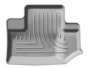
TO EASE INSTALLATION OF YOUR WRANGLER SECOND SEAT LINERS, FIRST MOVE BOTH FRONT SEATS TO THEIR MOST FORWARD POSITION. ONCE YOU HAVE INSTALLED YOUR LINERS, REPOSITION THE FRONT SEATS AS DESIRED.
