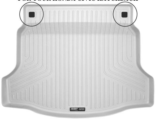
YOUR LINER, AS BOXED, COVERS THE FACTORY CARGO TIE-DOW HOOKS LOCATED NEAR THE REAR SEATS (SEE ABOVE CIRLCED). TO ACCESS THE CARGO HOOKS SIMPLY TRIM AWAY THE MATERIAL ABOVE THE HOOKS. TO AID IN TRIMMING THE AREAS ARE LOWERED. THE EDGE OF THE LOWERED AREA IS THE TRIMMING GUIDE. A UTILITY KNIFE OR SIMILAR WORKS WELL FOR TRIMMING.
