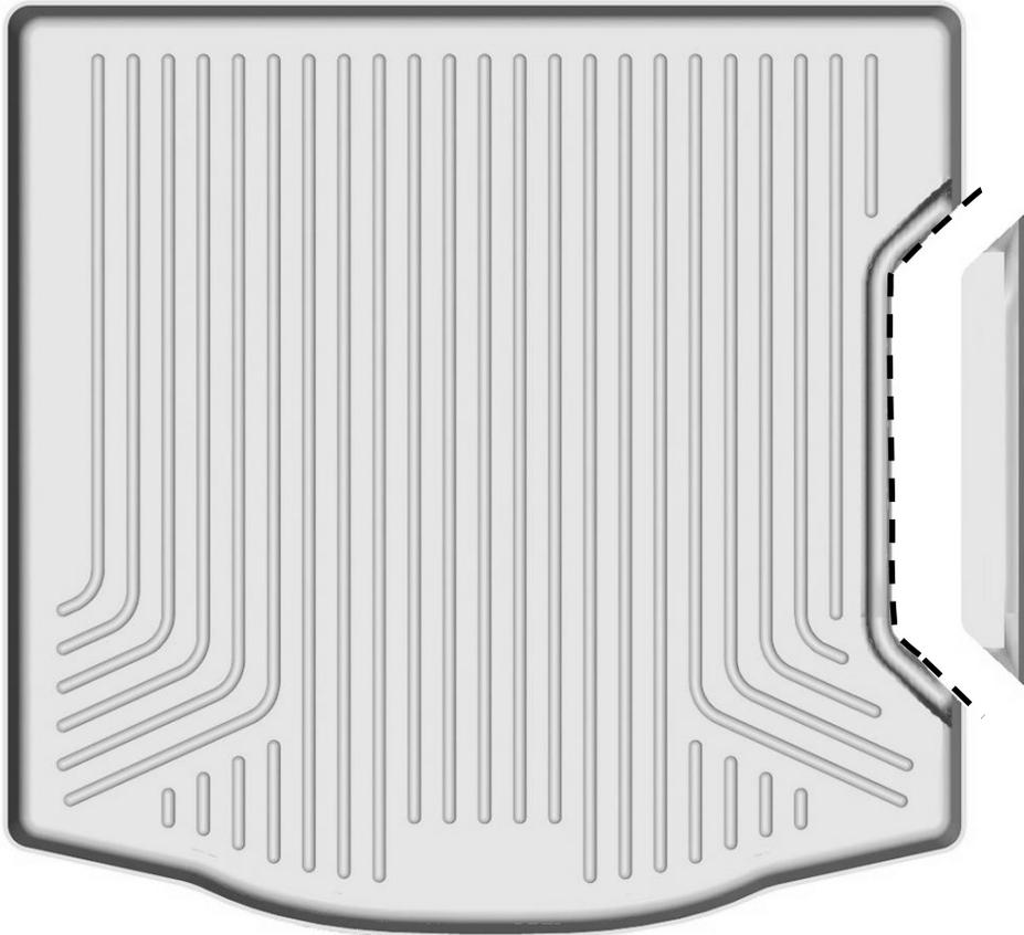
FOCUS MODELS EQUIPPED WITH THE OPTIONAL SONY AUDIO SYSTEM HAVE A SUBWOOFER MOUNTED IN THEIR TRUNK COMPARTMENT. THIS SUBWOOFER WILL KEEP YOUR LINER FROM FITTING AS IT IS BOXED. YOUR LINER IS DESIGNED TO ACCOMMODATE THE SUBWOOFER VIA TRIMMING. TO TRIM, FIRST LOCATE THE MOLDED IN STEP IN THE LINER THAT ACTS AS A TRIMMING GUIDE (SEE DIAGRAM ABOVE AND PHOTOS ON BACK OF PAGE). THEN, USING HEAVY
