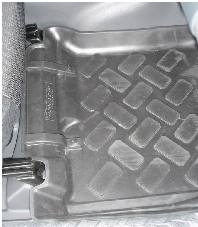
HUSKY LINER PART #3596 SHOWN INSTALLED IN THE FJ CRUISER. NOTE THAT LINERS MUST BE ATTACHED OVER FACTORY MAT HOOKS TO HELP SECURE LINERS IN POSITION.
