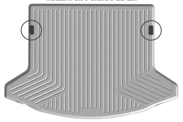
TO ACCESS THE FACTORY CARPET HOOK LOCATIONS WITH YOUR LINER IN PLACE, SIMPLY TRIM THE MATERIAL AWAY FROM THE AREAS DIRECTLY OVER THE HOOKS. THESE AREAS ARE SHOWN DARKENED/CIRCLED IN THE IMAGE ABOVE. USE THE LOWERED EDGES OF THE LOCATIONS AS YOUR TRIMMING GUIDE. A UTILITY KNIFE WORKS WELL FOR TRIMMING.
