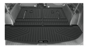
5. The first time the rear seat backs are moved to the upright position, move the seats slowly taking care to insure the accordion section of the liner folds outward as shown. This may need to be assisted from the backside.
