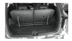
6. The liner at this point is fully installed and is ready to use. If the liner needs to be removed, grab the rectangular hook and loop fastener patches and hold them firmly in place as you pull the liner from the seat. This hook and loop fastener piece is intended to stay attached to the seat back and cargo floor to reduce ware from the liner being installed and reinstalled for cleaning.
