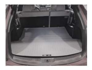
5. The first time the rear seat backs are moved to the upright position, move the seats slowly taking care to insure the accordion section of the liner folds outward as shown. This may need to be assisted from the backside.
