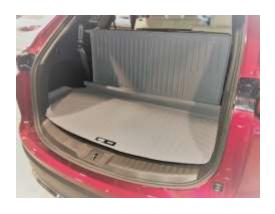
6. The liner at this point is fully installed and is ready to use. If the liner needs to be removed, grab the rectangular Velcro patches and hold them firmly in place as you pull the liner from the seat. This Velcro piece is intended to stay attached to the seat back and cargo floor to reduce ware from the liner being installed and reinstalled for cleaning.
